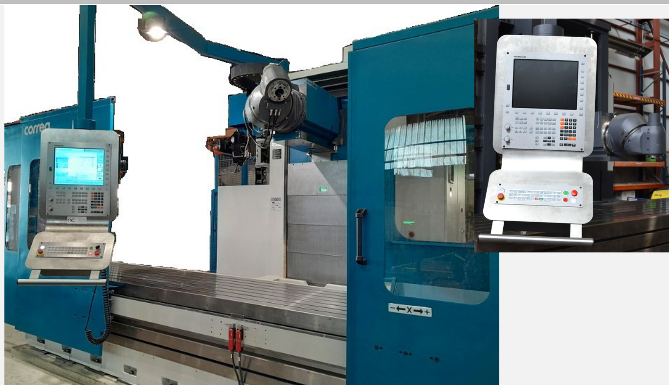
Example of a CORREA L30 milling machine after full retrofitting with new TNC-320
