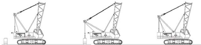
Unloading and assembly of counterweight
